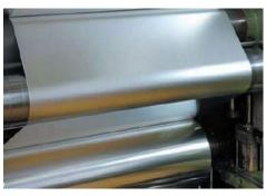
**Texobond F107** is a water-based heat seal coating for use in aluminum pouches. Unlike conventional heat seal coatings, Texobond F107 has excellent adhesion to metal surface which avoids 'stringing'. The coating has very good antiblocking properties and low coefficient of friction. The coating results in fiber tear seal strength when coated face to face.
